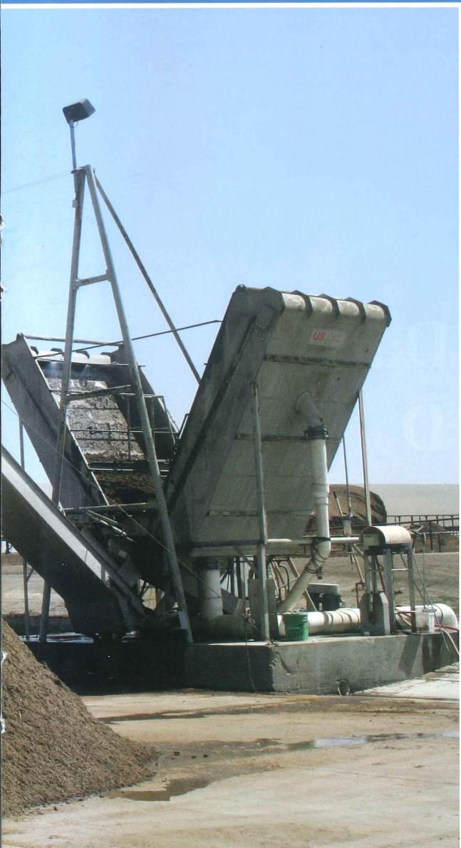
LARGE PHOTO: Manure separation is a preconditioning unit to composting. Manure separators remove three times as much manure as they did 10 years ago.
