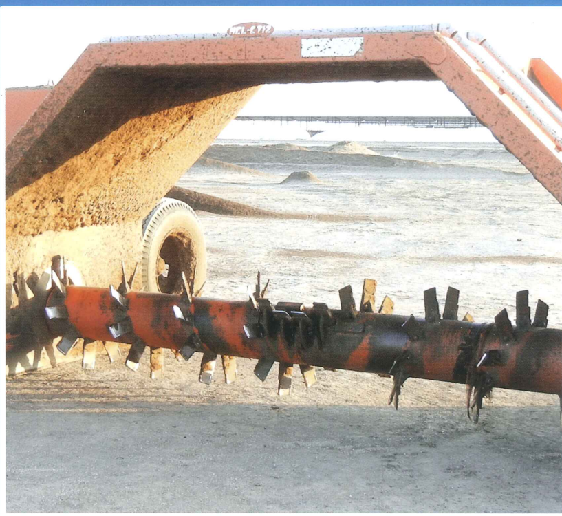
ABOVE PHOTO: The teeth on the compost turner perform mechanical agitation by mixing through the windrow.
