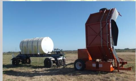
The hydraulically powered water pump is easily controlled within the cab of the tractor. Each water trailer is equipped with a polyurethane tank.
