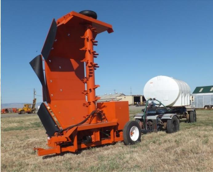
The HCL water trailer can be tailored to fit your specific application. The average capacity of our water trailers is between 2800-3000 gallons, and trailer frames vary depending on customer preference and stock on hand.
