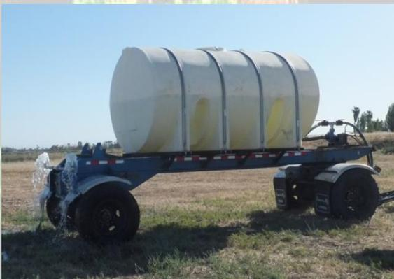
The HCL Water Trailer is equipped with rear facing water jets. The rear jets provide versatility as the trailer can be used to facilitate your dust control efforts.
