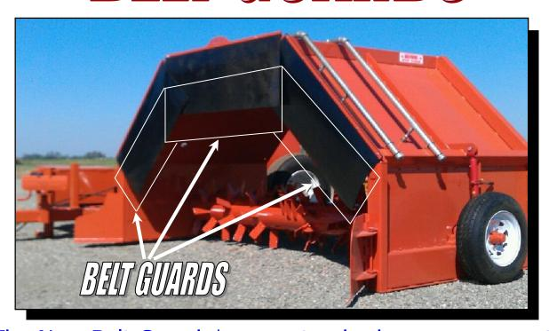
The New Belt Guards\*, now standard on our compost turners, are designed to block composting materials that may occasionally be projected forward during the composting process.
