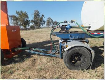
The HCL Water Trailer is equipped with rear facing water jets. The rear jets provide versatility as the trailer can be used to facilitate your dust control efforts.
