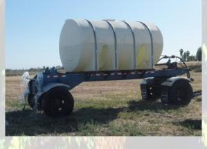
The HCL water trailer can be tailored to fit your specific application. The average capacity of our water trailers is between 2800-3000 gallons, and trailer frames vary depending on customer preference and stock on hand.
