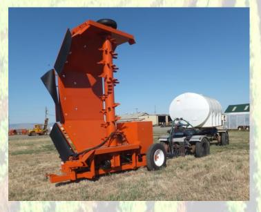
The hydraulically powered water pump is easily controlled within the cab of the tractor. Each water trailer is equipped with a polyurethane tank.
